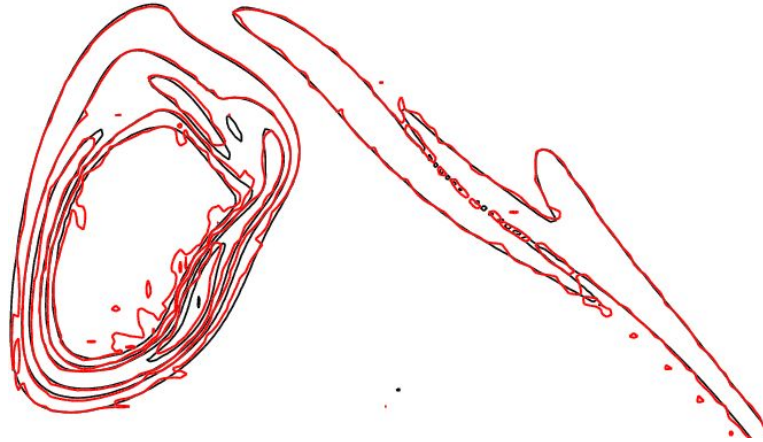
Figure 2. Iso-contours of the dimensionless vorticity norm. Comparison between the results obtained with PSM and DGM(4).
