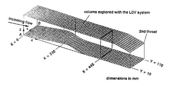
Figure 1: Geometrical definition of the three-dimensional channel (from [1])
